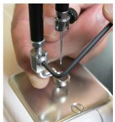
4. Ensure the middle of the foot opening is centered with the needle when the foot is fully tightened with the 2.5mm hex wrench. If it isn't properly centered, loosen the lock nut on the foot adaptor with an 8mm wrench, center the foot with the needle; hold the foot firmly in position; and tighten the lock nut.
