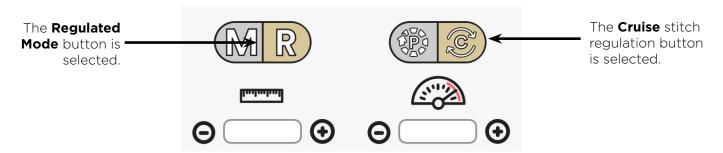
After pressing the **Start/Stop** button, the Start stitching indicator in the upper-left corner of the screen turns gold and the needle begins moving up and down according to the cruise speed or stitches-per-minute setting.
