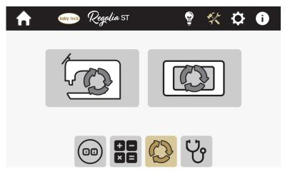
• After downloading the updated software to a USB drive, insert the drive in the designated USB port on the bottom of the front display. Look for the message in the bottom bar that confirms a USB drive has been inserted. If it doesn't appear, reinsert the USB drive. Touch the **Update** button. Press the **Home** button to return to the Main screen.
