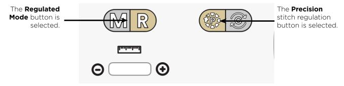
After pressing the **Start/Stop** button on the touchscreen, the fabric must be moved for the machine to begin quilting according to the stitches-per-inch setting. The Start button in the upper-left corner of the screen turns gold but the needle doesn't automatically begin moving up and down. Begin moving the fabric to begin stitching. Stitching pauses when the fabric is not moved and will start once the fabric is moved. To stop stitching, press the **Start/Stop** button on the touchscreen.
