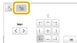
When rotating the pattern while checking the embroidering position shown by the camera, the embroidering starting position can be set using a mask based on the pattern before it has been rotated, which is useful for aligning. (page 75)
