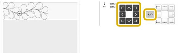
Then, align the end point of the last pattern with the start point of the first pattern. If the pattern is not angled correctly, rotate it. If the length of the pattern does not match, enlarge or reduce the pattern.
