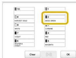
3 Touch the number of the other needle bar that will be switched. The two needle numbers are connected with an arrow.
