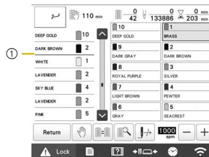
① indicates when the thread spools will need to be changed. The thread spools will need to be changed the number of times that this indicator is displayed and between the two thread colors at the point where it is displayed.
