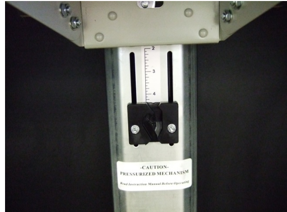
4-1/2" machine in Arrow place 4-3/8" mark
