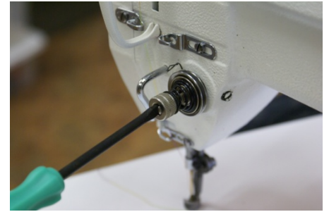
Fig 27: For fine adjustment of check spring insert screwdriver turn clockwise for more tension
