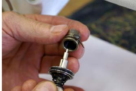
Fig 17: Insert the tension assembly back in barrel
