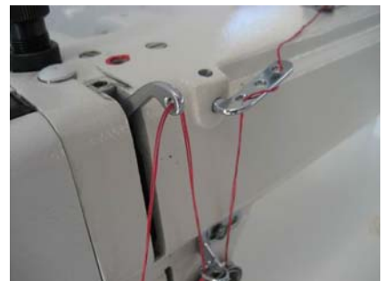
Takeup lever guard removed for photos only. Never run the machine without the guard in place, extreme head injury may occur.
