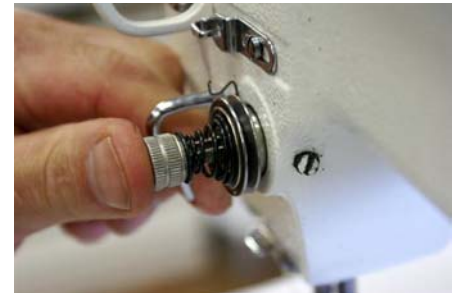
Fig 24: Release and the disk will close; this is the proper place for your tension assembly
