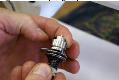
Fig 19: give the tension assembly a twist until you feel resistance on the check spring
