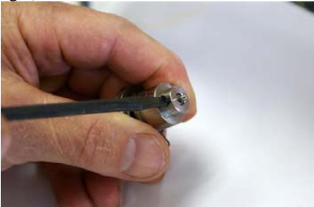
Fig 7: Loosen screw only DO NOT REMOVE
