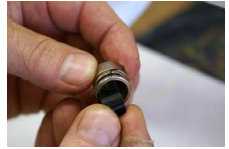
Fig 15: Twist while inserting new spring
