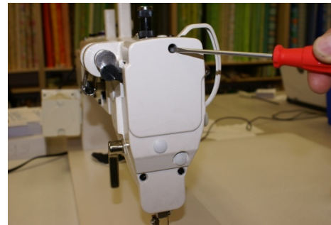
You will also need to remove the three Face plate screws
