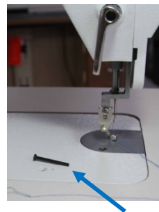
Oil Reservoir with dip stick removed
