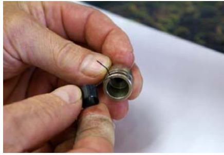
Fig 14: Insert New Spring
