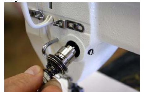
Fig 21: Place the assembly back into your machine
