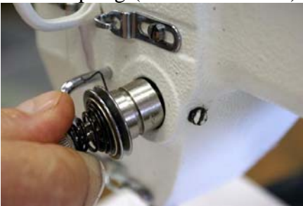
Fig 4: Remove assembly from machine. Be careful of release pin (see fig 6)
