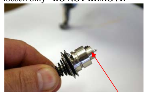
Fig 6: Tension assembly out of machine DO NOT LOOSE PIN
