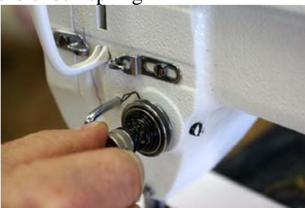
Fig 22: Once in ensure that your check spring is at 11:00 (refer to fig 26 for correct placement)
