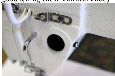
Fig 5: Machine with tension assembly removed
